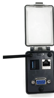
No.4: Tighten the screw and close the waterproof cap
