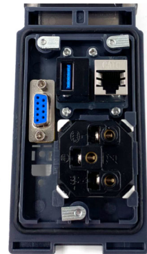
No.2: Remove the screw waterproof cap Loosen the screw
