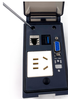
No.2: Remove the screw waterproof cap Loosen the screw
