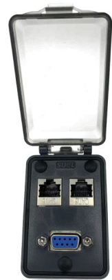
No.4: Tighten the screw and close the waterproof cap
