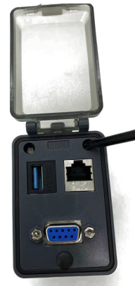
No.4: Tighten the screw and close the waterproof cap
